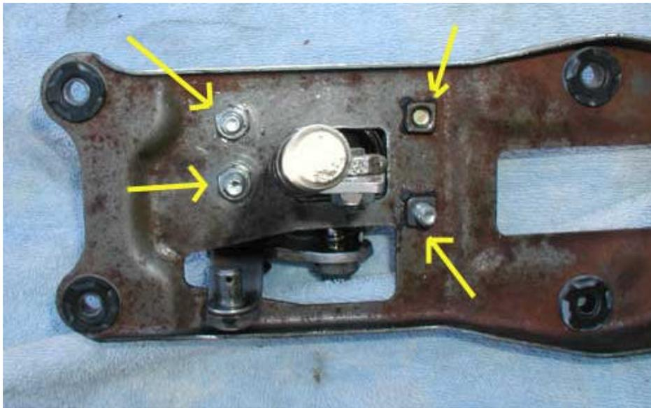
4. Note the position of the lower shift lever pivot with regards to the neutral return spring before removing the lever from the shifter.
