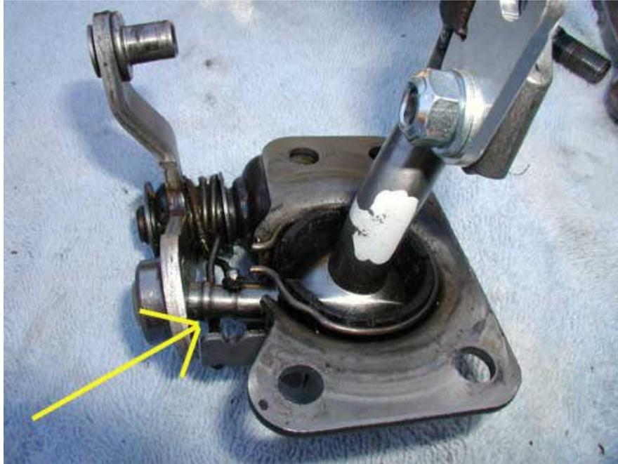
5. Remove the lever by pulling it up and twisting the lower arm free of the neutral return spring.
