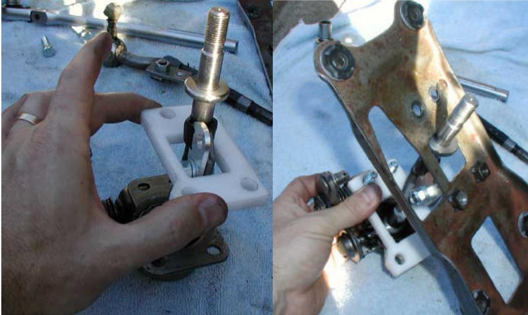
8. Install the lever assembly using the three longer bolts and one of the original bolts. The short bolt goes in the rear, right side hole.
